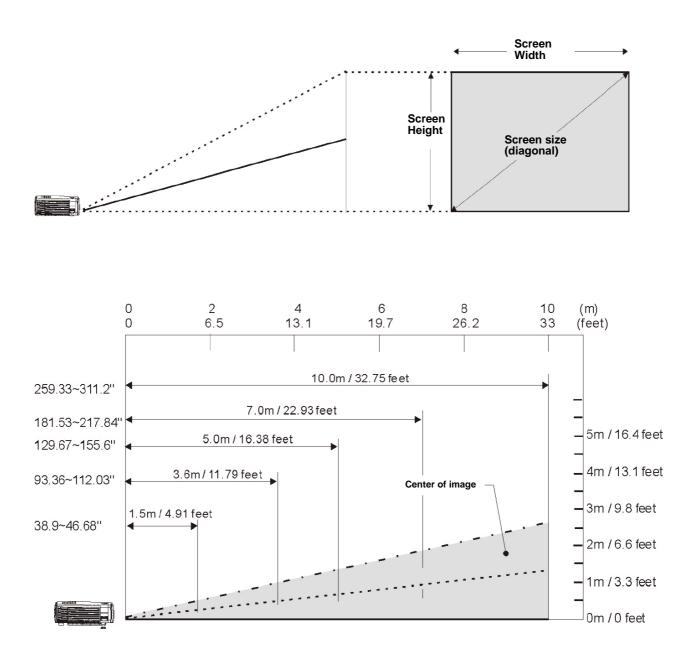
Figure 1: Projection Distance vs. Image Size
